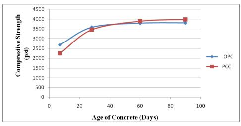
Fig. 6: Compressive strength (Psi) Vs Age of Concrete (Days) Mix ratio 1:1.5:3, water cement ratio: 0.45.
