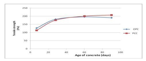
Fig. 9: Tensile strength (Psi) Vs Age of Concrete (Days) Mix ratio 1:2:4, water cement ratio: 0.6.
