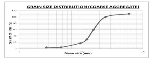
Fig. 2: Grain size distribution curve of coarse aggregate (Gas burn brick).
