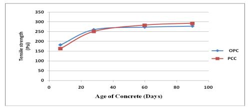
Fig. 8: Tensile strength (Psi) Vs Age of Concrete (Days) Mix ratio 1:1.5:3, water cement ratio: 0.45.
