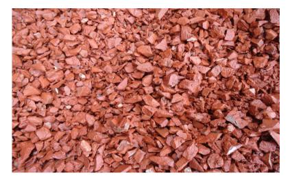
Fig. 3: Photo view of 1<sup>st</sup> class brick aggregate used as coarse aggregate.
