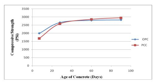
Fig. 7: Compressive strength (Psi) Vs Age of Concrete (Days) Mix ratio 1:2:4, water cement ratio: 0.6.
